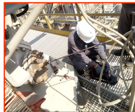
Stack Emission Testing
