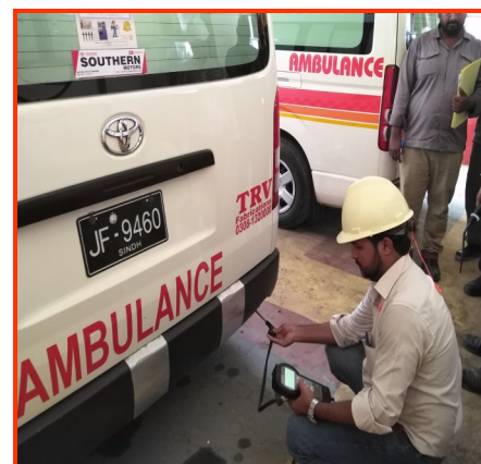
Vehicle Emission Monitoring
